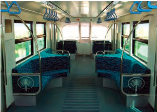
Fig. 3—Design of Front End of Monorail Vehicle. Sightseeing seats that give passengers a good view of the surroundings are located at the front end of the monorail vehicles while the mid-sections of the vehicles are fitted with round seats where passengers can relax.
