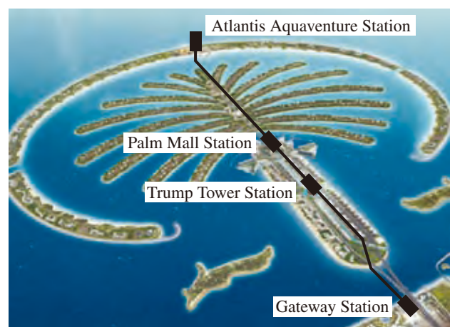
Fig. 1—Palm Jumeirah Transit System Track Map. The line runs from Gateway Station on the mainland to Atlantis Aquaventure Station at the far end of the island, with intermediate stations at Trump Tower and Palm Mall where high-rise buildings and shopping malls respectively are planned for construction.
