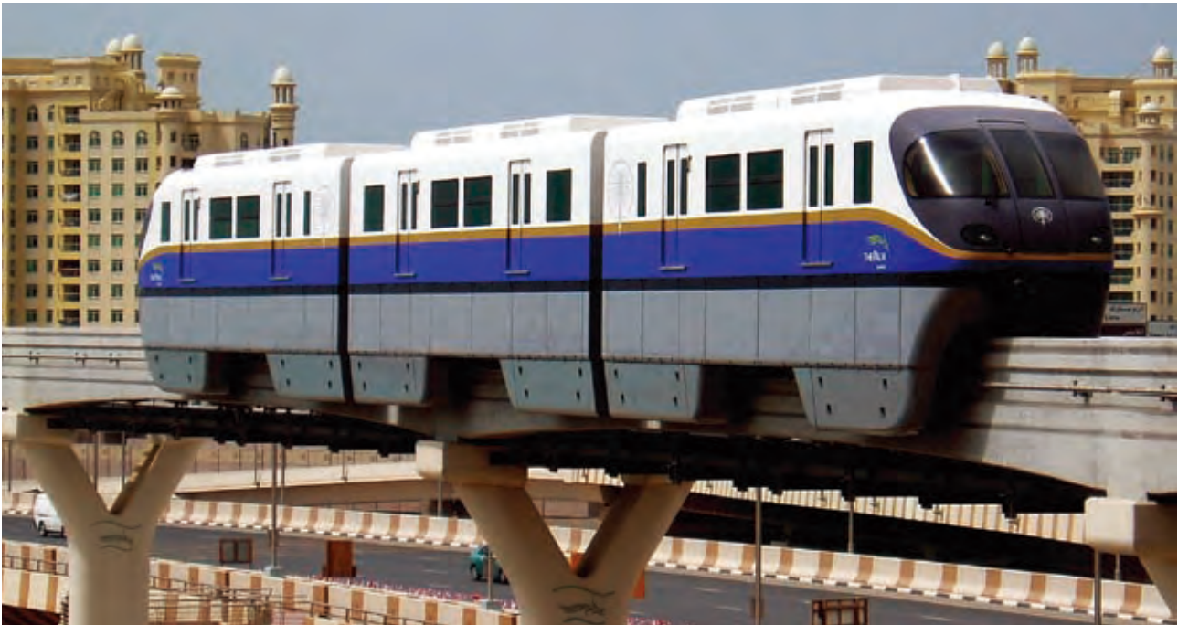
Fig. 2—Monorail Vehicle for Palm Jumeirah Transit System. The monorail vehicles are the first to use a double-skin structure based on the A-train concept.
