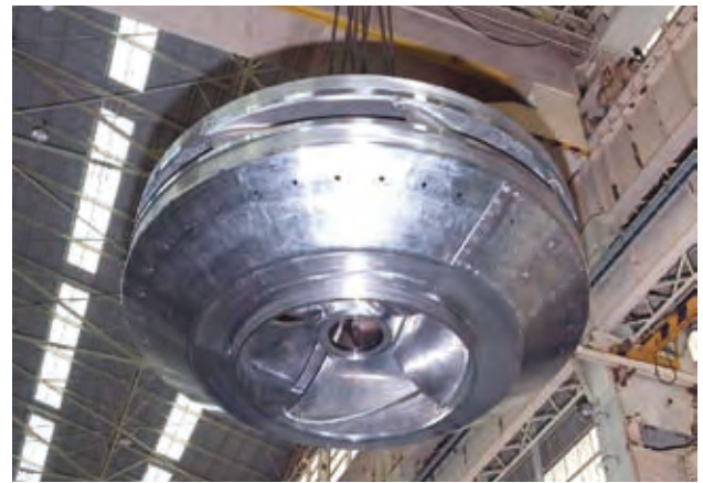
Fig. 7—Manufacture of Pump-turbine Runner with Intermediate Vanes for Okutataragi Power Plant of Kansai Electric Power.
