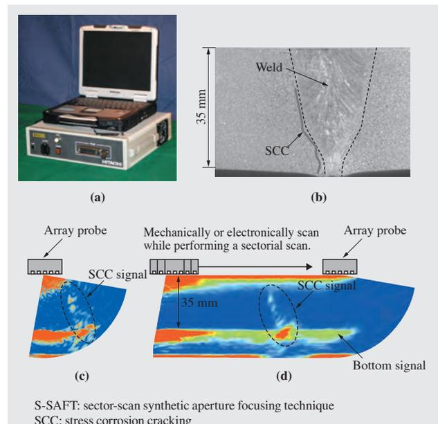
Fig. 1—Phased Array Ultrasonic Testing System and Example Test Images.
