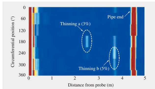
Fig. 5—Example Measurement of 500 A Pipe Using Partially Attached Probe.
