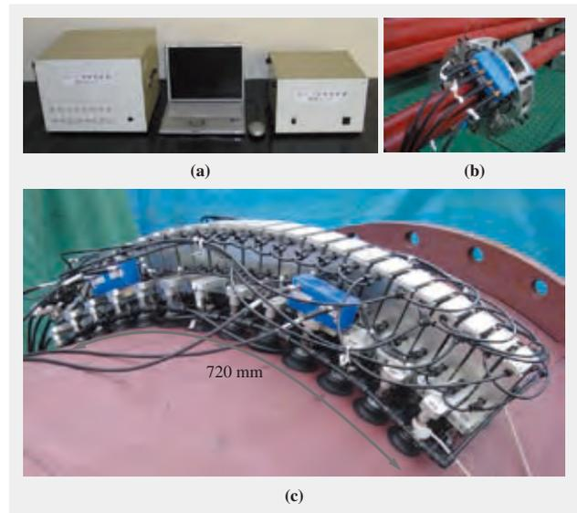
Fig. 4—Portable Guided Wave Inspection System. Guided wave transceiver unit (a), probe for 50 A pipes (b), and partially attached probe for large-diameter pipes (c) are shown.
