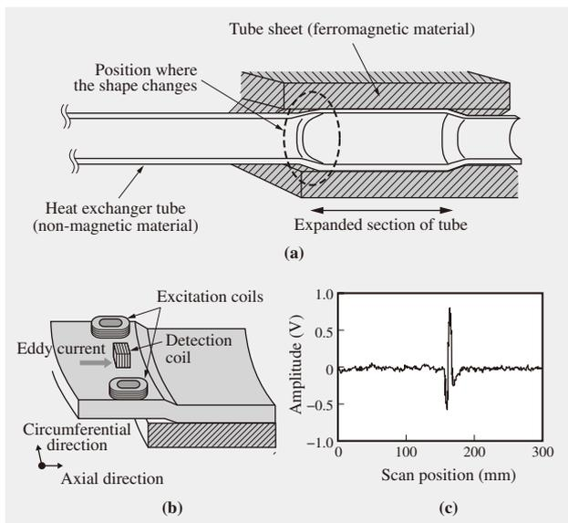
Fig. 6—Eddy Current Testing System for Inspecting Heat Exchanger Tubes.
