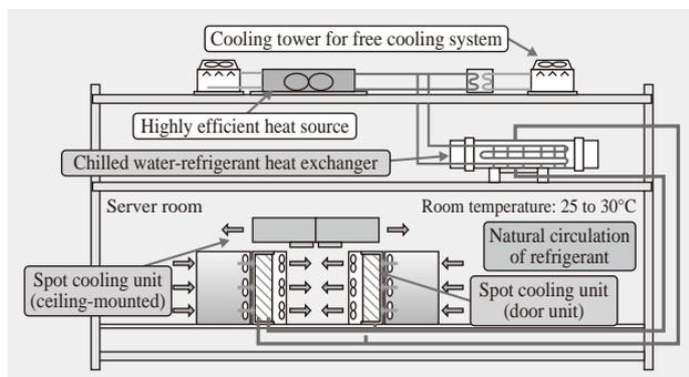
Fig. 3—Overview of Spot Cooling System with Natural Circulation of Refrigerant.
