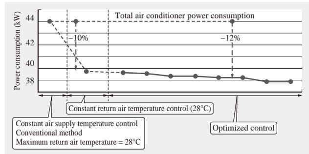
Fig. 7—Air Conditioning Power Savings Achieved by Controlling Air Conditioning based on IT Power Consumption. Compared to constant air supply temperature control used previously, constant return air temperature control reduces air conditioner power consumption by 10% and optimized control reduces power consumption by 12%.
