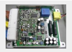
Fig. 7—Integrated Battery Controller for Hybrid Vehicle Battery System.
