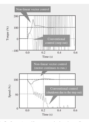
Fig. 7—Comparison of Responses to the Out-of-range External Impact Load by Motor with Highly Non-linear Characteristics (Simulation).
