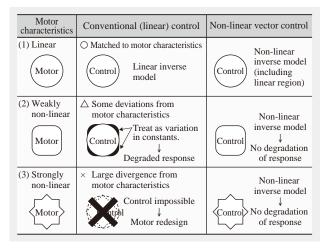
Fig. 6—Concepts of Linear and Non-linear Control Based on Motor Characteristics.
