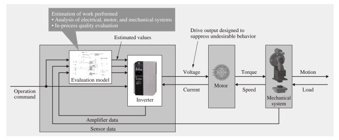
Fig. 11—Use of Evaluation Model of Mechanical System to Enhance Control Performance. The evaluation model is used to estimate the work performed by the motor, analyze individual components, and review the quality of machining operation. This information is used when operating the motor to enhance the drive unit by making changes such as varying the drive torque and switching operation mode.
