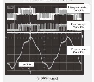
PWM: pulse width modulation HEV: hybrid electric vehicle
