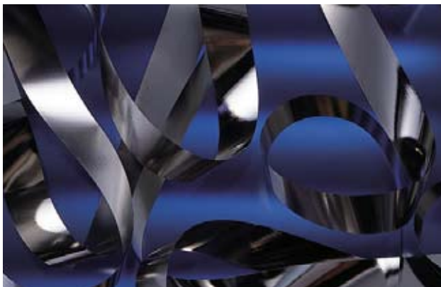
Fig. 6—Amorphous Ribbon. This wide Fe-based amorphous ribbon is produced using a melt spinning process with excellent productivity.
