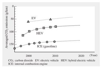
Fig. 1—Projections for Average Automotive  $CO_2$  Emission Levels (Survey by Hitachi Research Laboratory). HEVs and EVs have progressively greater potential for reducing vehicle  $CO_2$  emissions.
