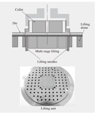
Fig. 2-New Lifting Mechanism.
