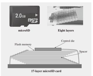
Fig. 3—External View and Interior Structure of Memory Card. A photograph of a microSD card, a SEM (scanning electron microscope) image of its interior (eight layers), and a diagram of its structure (17 layers) are shown. Bonding a large number of identical dies together in a single package allows higher memory capacities to be achieved.
