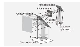
Fig. 4—Configuration of Exposure Projection System. The light from the light source is reflected by the first flat mirror onto the fly's-eye lenses and then travels via the concave lens and final flat mirror to be projected onto the mask in the form of parallel rays.
