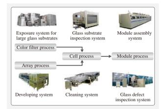
Fig. 1—Production Process and Equipment Range for LCDs. TFT (thin film transistor) LCD (liquid crystal display) production consists of four processes, namely the color filter, array, cell, and module processes. Hitachi High-Technologies Corporation supplies manufacturing and inspection equipment for each of these processes.
