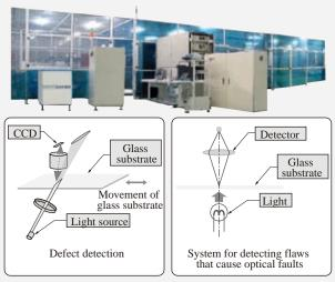
CCD: charge-coupled device
