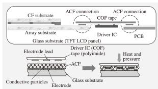
CF: color filter ACF: anisotropic conductive film COF: chip on film IC: integrated circuit PCB: printed circuit board
