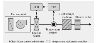
Fig. 5—Air Conditioning System with Precise Temperature Control. Characteristics include a quick-acting heater, minimization of temperature fluctuations through use of heat storage medium, and other techniques.
