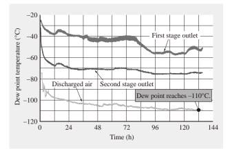
Fig. 11—Change in Air Dew Point Temperature over Time. The graph shows operating data for the super clean ultra-low dew-point air generator system at startup. The results demonstrate the excellent dehumidification performance of the system, with the dew point of the discharged air reaching  $-100^{\circ}C$  after 20 hours and  $-110^{\circ}C$  after 6 days.
