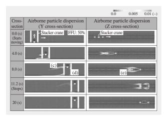
Fig. 4—Analysis Results for Airflow and Airborne Particle Dispersion when Local Ventilation Used to Improve Cleanliness.
