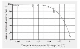
Fig. 12—Relationship between Dew Point Temperature and Organic Compound Removal Performance. The performance at removing organic compounds improves as the dew point falls, reaching better than 99% removal when the
