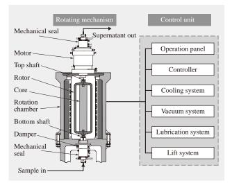
Fig. 2—Structure of Rotating Mechanism and Control Unit. The centrifuge is driven by a high-frequency motor. The sample is introduced via the bottom mechanical seal, separation takes place inside the rotor, and then the supernatant (leftover material) is discharged from the top mechanical seal.
