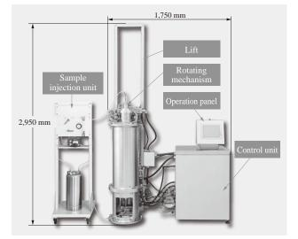
Fig. 5—Hitachi CC40NX Continuous Flow Ultracentrifuge. First released in October 2009, the ultracentrifuge has a maximum speed of 40,000 min<sup>-1</sup> and numerous features including support for steam sterilization of the sample flow path and electronic recording of operating data.
