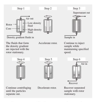
Fig. 4—Operating Procedure for Continuous Flow Centrifugation. Continuous flow centrifugation forms a density gradient in the fluid inside the rotor. This causes the target material to separate out in the density gradient band from which it can be recovered. into the rotor from the bottom shaft. The buffer is a solution in which the concentration of hydrogen ions has been adjusted to prevent loss of activity by the biological sample.
