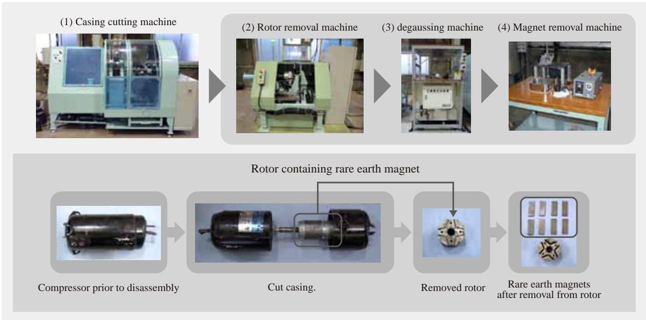
Fig. 4—Process for Recovering Rare Earth Magnets from Compressors.
