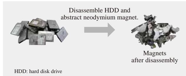
Fig. 2—Recovery of Rare Earth Magnets from HDDs. In the past, HDDs needed to be disassembled manually to collect the rare earth magnets because the magnets are difficult to recover if crushed.
