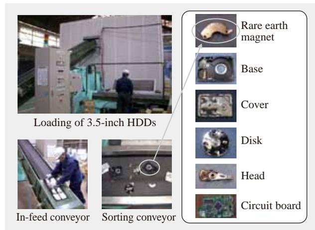
Fig. 3—Overview of HDD Disassembly Machine. The HDDs are loaded into the machine via an in-feed conveyor where they are disassembled into their component parts and ejected. The parts are sorted on the conveyor and collected individually.
