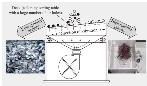
Fig. 10—Specific Gravity Sorting Machine for Mixed Plastics. The machine uses air pressure and vibration to sort materials with different specific gravities based on the difference in frictional force.
