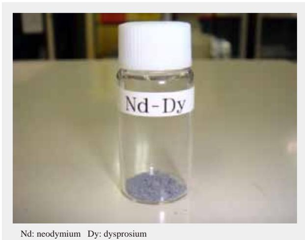
Fig. 5—Rare Earth (Nd, Dy) Alloy Abstracted from Magnets. The rare earth alloy shown here was recovered by melting together with an abstraction medium with a strong affinity for rare earths and then raising the temperature to evaporate the abstraction medium.
