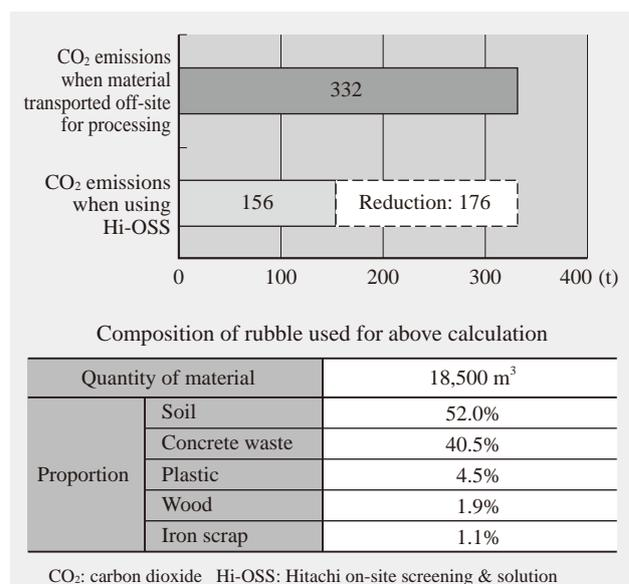
Fig. 6—Comparison of CO<sub>2</sub> Emissions when Material Transported Off-site for Processing versus Using Hi-OSS. The figure shows a comparison of CO<sub>2</sub> emissions when material transported to an off-site processing facility versus performing similar processing on-site.
