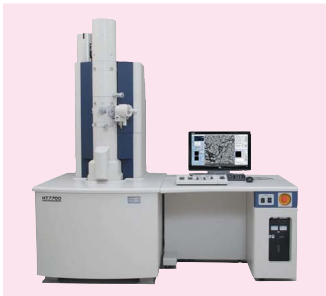
HT7700 transmission electron microscope
