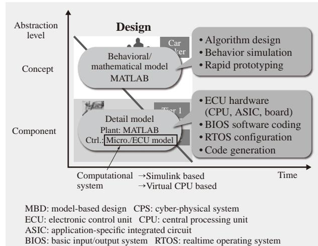
Fig. 2—V-cycle Incorporating MBD and CPS Approach.
