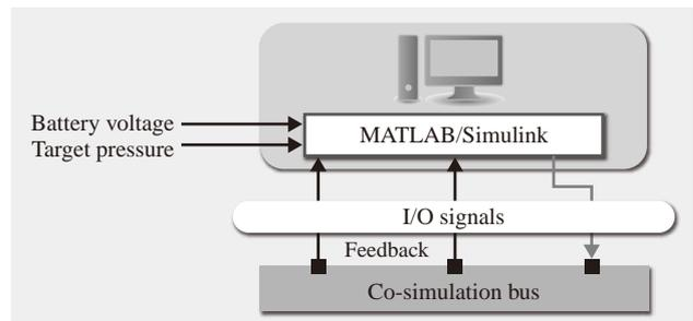
Fig. 6—Gasoline Fuel Pump Computational System. The simulation model of the gasoline fuel pump control system interfaces to a co-simulation bus.
