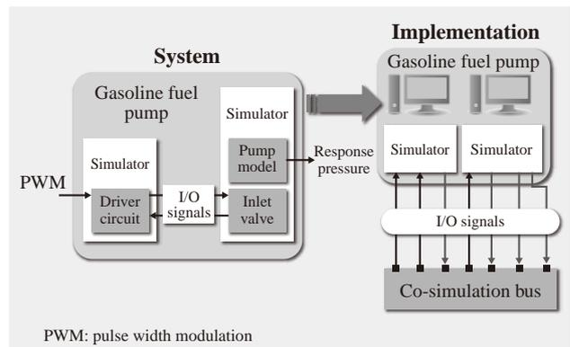
Fig. 5—Gasoline Fuel Pump Physical System. This block diagram of the gasoline fuel pump system and its simulation model represents a multi-PC implementation with a co-simulation bus.
