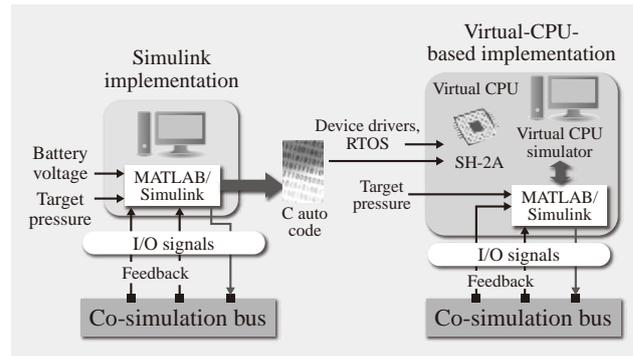
Fig. 8—Auto-code Generation for SH-2A CPU. The Simulink-based control model was converted into C code, compiled with the device drivers and RTOS, and executed on the Renesas Electronics Corporation's SH-2A CPU.
