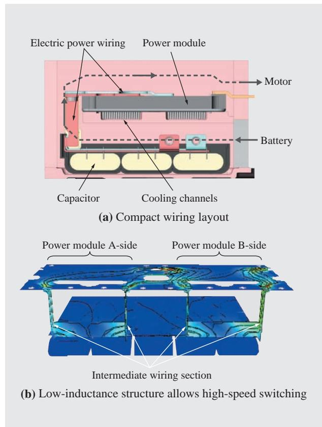
Fig. 3—Wiring Layout and Low-inductance Structure of Next-generation Inverter. The inverter consists of three areas with cooling water channels running down the center. The design significantly reduces the area required for wiring by providing a compact flow of electric current in the housing. It also provides more flexibility for attaching external connections, and reduces inductance by controlling the current density distribution in the intermediate wiring section.
