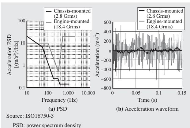
Fig. 6—PSD Representing Intensity at Each Frequency of Random Wave, and Example of Actual Acceleration Waveform. The vibrations to which an inverter is subject differ significantly depending on factors such as where it is mounted, whether the vehicle has an engine, the engine type, and suspension performance.
