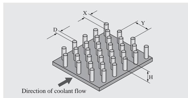
Fig. 4—Definition of Heat Sink Design Variables with Respect to Direction of Coolant Flow.
