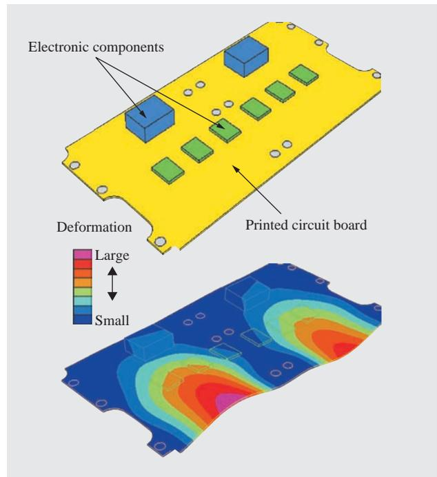
Fig. 7—Vibration Analysis of Inverter Printed Circuit Board. Used in conjunction with three-dimensional computer-aided design (3D-CAD) software, the technique provides a designer working at a desktop with a workflow that proceeds from shape design to analysis and then uses the assessment results as feedback to the shape.
