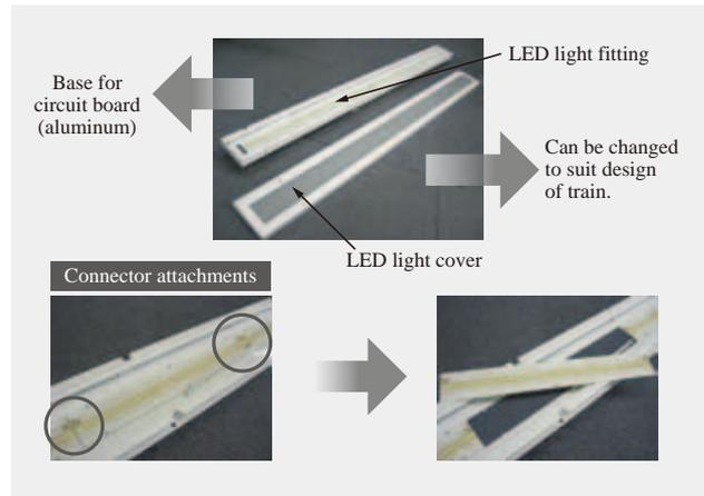
*Fig. 3—LED Light Design and LED Circuit Board.*
