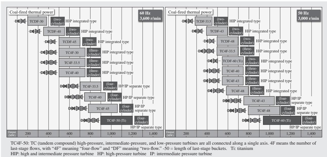
Fig. 3—Output Lineup of Steam Turbines for Use in Coal-fired Power Generation, Based on Turbine Type and Last-stage Blade Length. These 50-inch and 60-inch blades are used in 1,000-MW class output steam turbines with low-pressure turbines and two cylinders (four flows).
