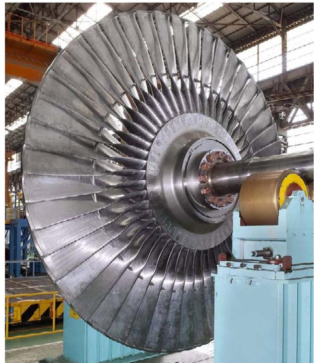
*Fig. 1—3,600 r/min 50-inch Last-stage Buckets. With an annulus area among the largest in the world<sup>\*2</sup>, turbine efficiency is improved by reducing wasted kinetic energy.*
