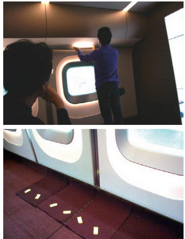
Fig. 7—Full-size Interior Mock-up Used to Evaluate Design. The mock-up was used to conduct an overall evaluation and verification of the interior design, lighting effects, compatibility between interior materials and the seating, and the sense of high quality conveyed by the space.
