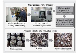
Fig. 3—Process Used to Separate and Recover Rare-earth Magnets from Air Conditioners.
