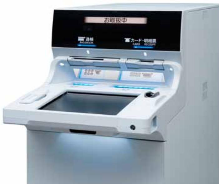
*Hitachi finger vein authentication system. The system is used for personal identification at bank ATMs.*
