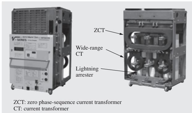
Fig. 9—Overview of All-in-one Hybrid VCB. Maintenance is facilitated by fitting the CT and lightning arrester in the drawer-mounted hybrid VCB so that they can be pulled out for inspection along with the VCB.
