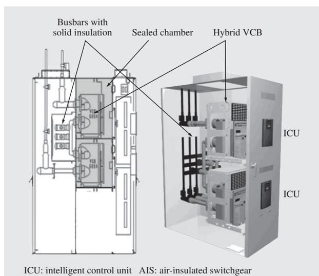
Fig. 8—Layout of 7.2-kV Panel with Solid Busbar Insulation. The solid busbar insulation and use of a sealed chamber to house the VCB overcome the problems associated with previous AISs.
