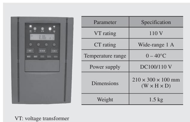
Fig. 12—ICU Photograph and Specifications. Use of the multifunction multi-relay helps make switchgear smaller by integrating the wide-range CT.
