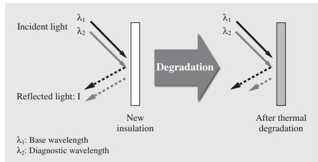
**Fig. 4—Principle of Operation of Dual-wavelength Optical Diagnostic Technique.**
