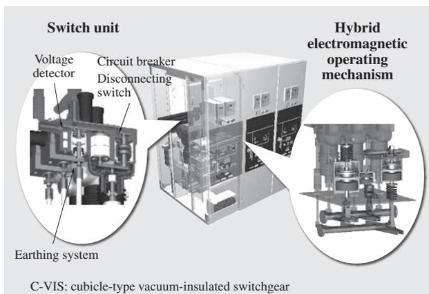
Fig. 10—Overview of 24-kV C-VIS. Hitachi has developed a switchgear based on a new concept that combines a hybrid electromagnetic operating mechanism with a multifunction vacuum interrupter. In addition to existing markets, Hitachi has also started supplying these for use in harsh environments such as in tropical regions and at sea.
