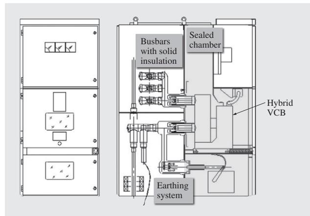
Fig. 14—Panel with Solid Busbar Insulation for Overseas Markets. Hitachi sells panels with solid busbar insulation in the Japanese market and is now considering expanding into the high-end market overseas.
