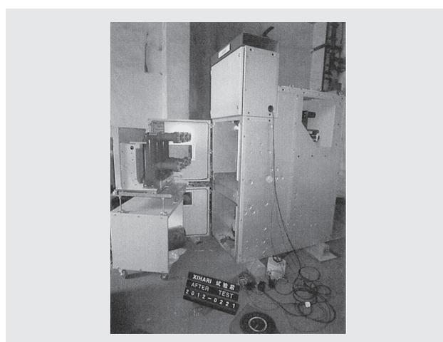
Fig. 7—Certification Testing of 12-kV Hybrid VCB for the Chinese Market. After testing, the supplied VCB was inspected to ensure it had no problems.
