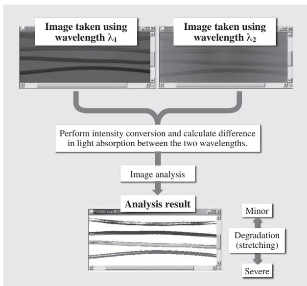
Fig. 5—Use of Dual-wavelength Optical Technique to Assess Cable Degradation. The technique is used to assess degradation of electric cables.
