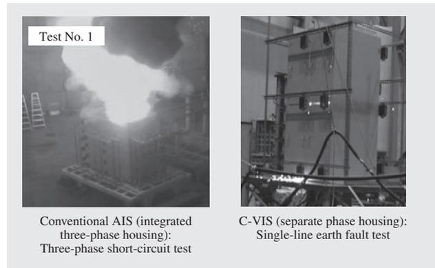
Fig. 11—Internal Arc Testing of Switchgear. Use of a design in which the phases are kept separate significantly reduced the consequences of internal arc accidents.
