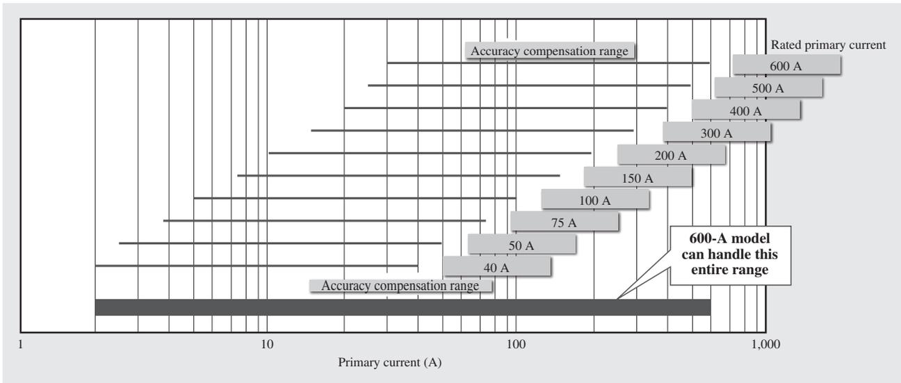
Fig. 13—Comparison of Current Compensation Ranges for Wide-range CT and Previous CT. The wide-range CT has a wide performance compensation range, reducing the need to replace the CT to handle higher loads.
