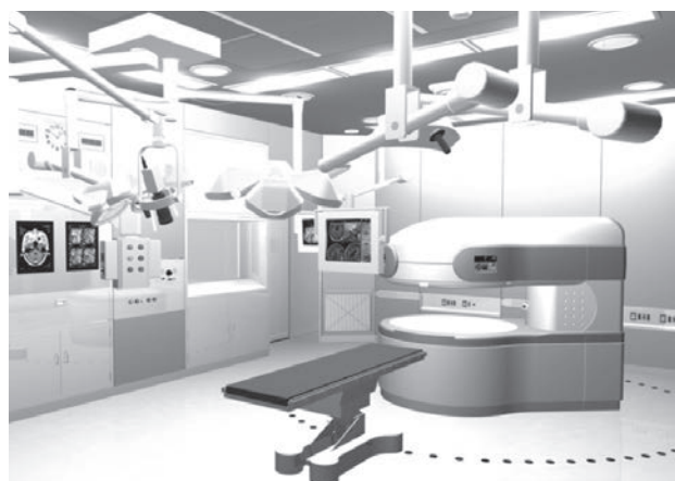
Fig. 2—Use of MRI as an Intraoperative Imaging System. A neurosurgery operating theater equipped with an open MRI system. The dotted line on the floor indicates the magnetic field safety zone with a threshold of 0.5 mT (approximately 10 times the Earth’s magnetic field). Conventional surgical instruments can be used outside this zone.
