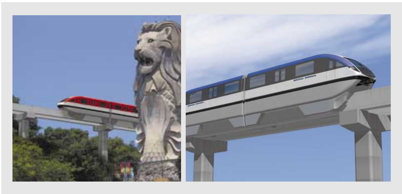
Fig. 1—Image of Sentosa Express (New Monorail System) Operating in Singapore. Based on decades of experience with larger monorail system technologies, Hitachi has developed a small, standard and cost-effective straddle-type monorail system to meet the transportation needs of small to medium-sized cities.
