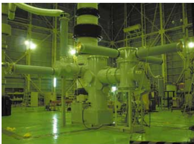
Fig. 6—Withstand Voltage Test on GIS.
