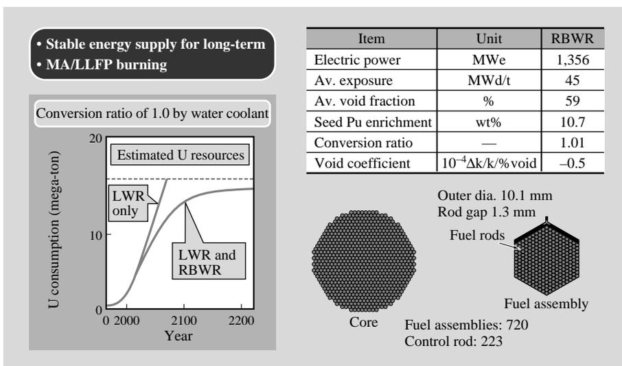
Fig. 4—Typical RMWR Concept (RBWR). Fuel rods are arranged tightly with a hexagonal fuel lattice configuration, and this is ideal for reduced moderation.
