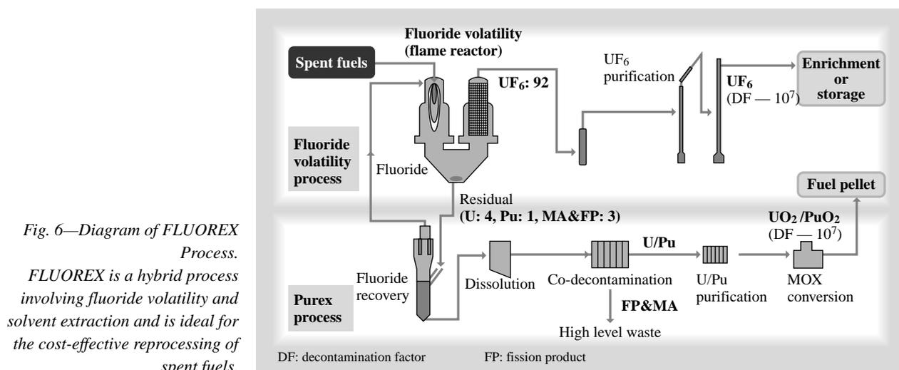
Fig. 6—Diagram of FLUOREX Process.
