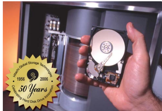
Fig. 2—First Hard Disk Drive with 24" Diameter Disks Compared with Modern 2.5" HDD.
