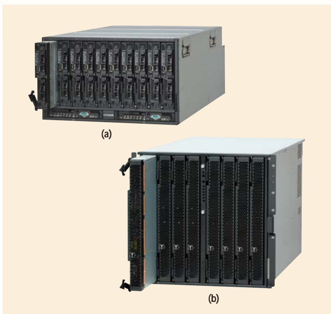
6U high-density blade server (a) and 10U high-end blade server (b)
