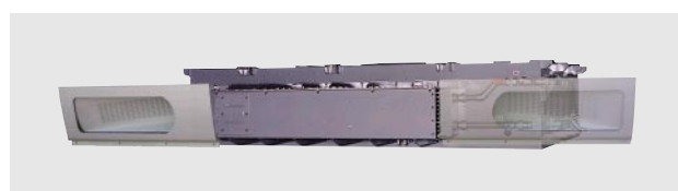
Fig. 3—External Appearance of the Main Converter of the Water-cooling System Utilizing Air-flow during Train Running. By fitting a water-cycle-cooling system using airflow generated during train running (thereby eliminating the need for electrical air circulation), a compact, lightweight, and low-noise main converter was accomplished.
