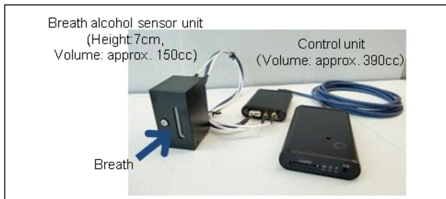
Prototype breath alcohol detection system
