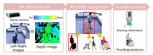
Estimation of attributes by analyzing 3D data obtained from a stereo camera and examples of services
