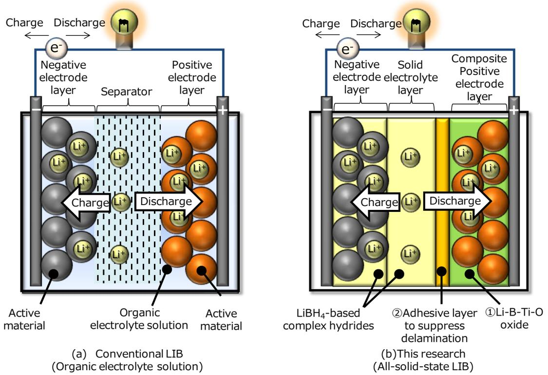
Fig.1 Schematic illustration of lithium ion battery (LIB)
