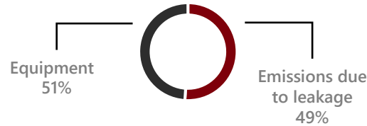
Cost of the Ownership: SF 6 420 kV GIS*
