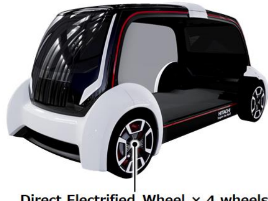
Fig. 2 Electric vehicle (mock-up) with direct-drive system installed inside wheel
