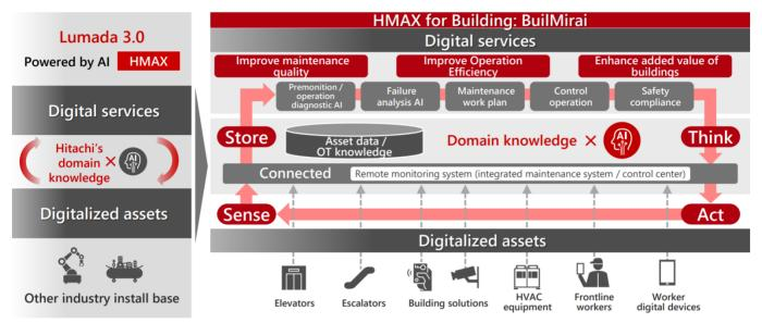
HMAX for Building: BuilMirai to provide value as a digital service that combines digitalized assets with knowledge and Al
