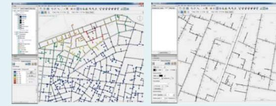
Pressure distribution simulation    Flow direction display simulation
