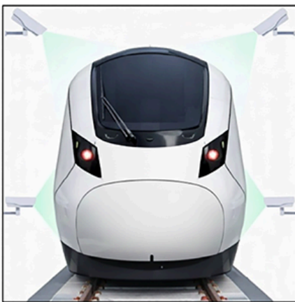
Camera installation for roof and side inspection
