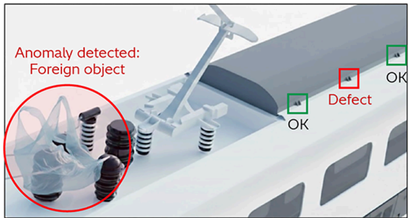
Inspection result: Detected defects and anomalies are highlighted and explained.
