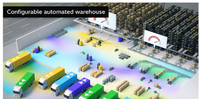
New practice: Different types of transport equipment operate in the same area Inbound and outbound goods handling share floor space and equipment, achieving higher utilization workloads
