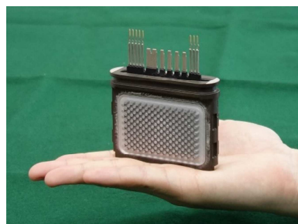
Direct water-cooling type double-sided cooling power module
