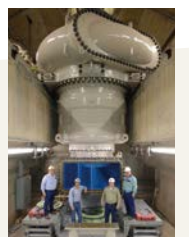
2011 Large-scale centrifugal pump with the world's highest efficiency level, supplied to Edmonston pumping station, USA.
