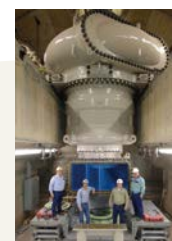
2011 Large-scale centrifugal pump with the world's highest efficiency level, supplied to Edmonston pumping station, USA.
