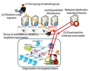
Figure 4: Watering Hole Attack.
