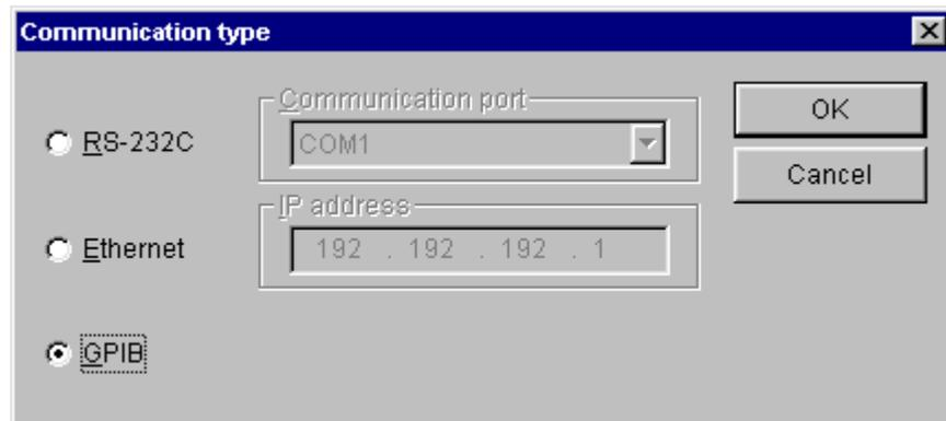
Figure 3-28 [Communication type] Window (GP-IB Connection)
