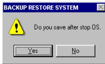
Figure 3-5 [BACKUP RESTORE SYSTEM] Dialog Box (OS Stop Confirmation)
