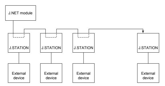
• When the J.NET module is connected to J.STATIONs (data transmitted)
