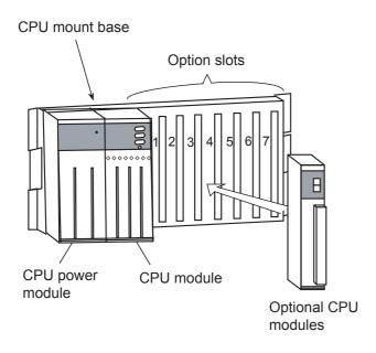
CPU extension mount base: HSC-1080 PS slot: Slot into which the CPU power supply (LVQ000) is inserted.
