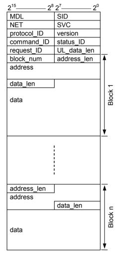
MDL: Module No. (= /00 for main module; = /01 for sub-module)
