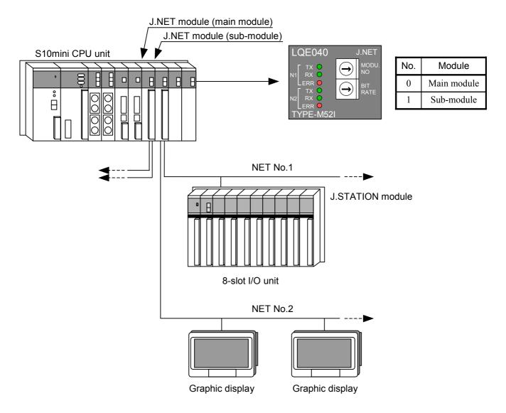
When using only one J.NET module, be sure to set it up as the main module. When using two J.NET modules, be sure to set up one module as the main module and the other as the sub-module.
