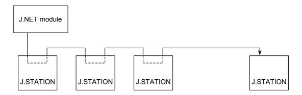
J.STATIONs are mounted on an I/O unit to constitute a remote I/O unit.
