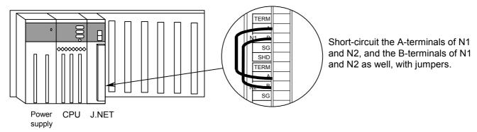
• T/M No.7 (cabling is performed as shown in the figure below)
