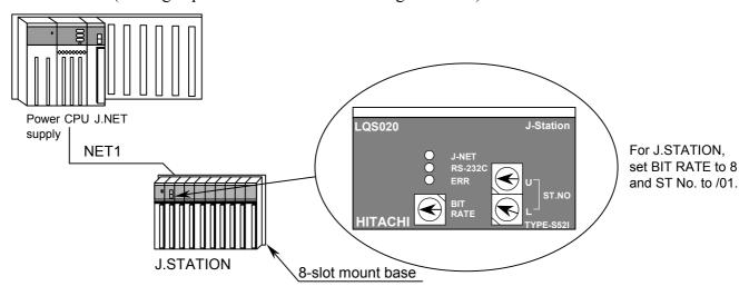
• T/M No.8 (cabling is performed as shown in the figure below)
