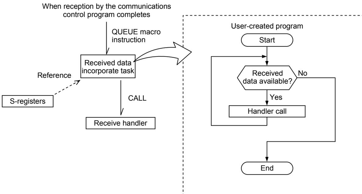
Figure 5-3 Incorporating Received Data with an Application Task (C Mode)
