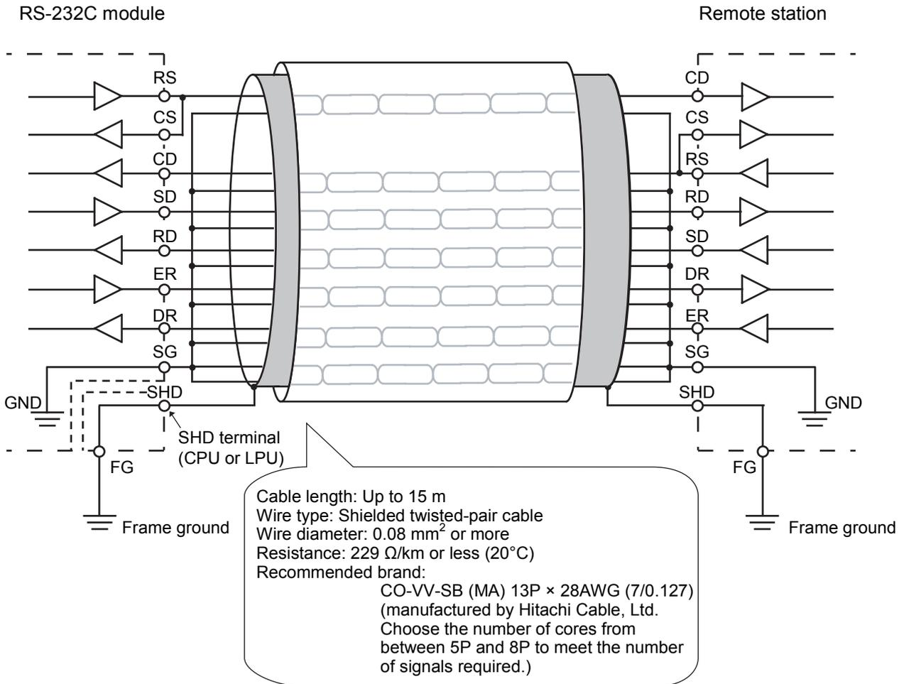
Figure 3-3 Example of RS-232C Wiring
