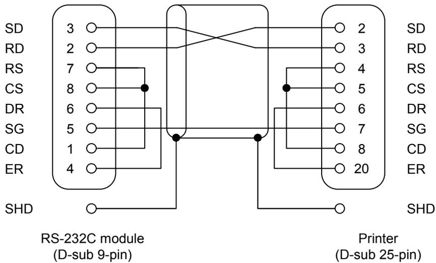
Figure 5-5 RS-232C Signal Connections
