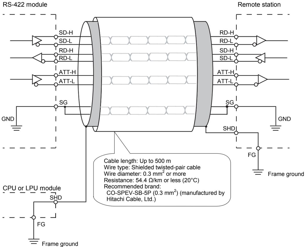
Figure 3-4 Example of RS-422 Wiring
