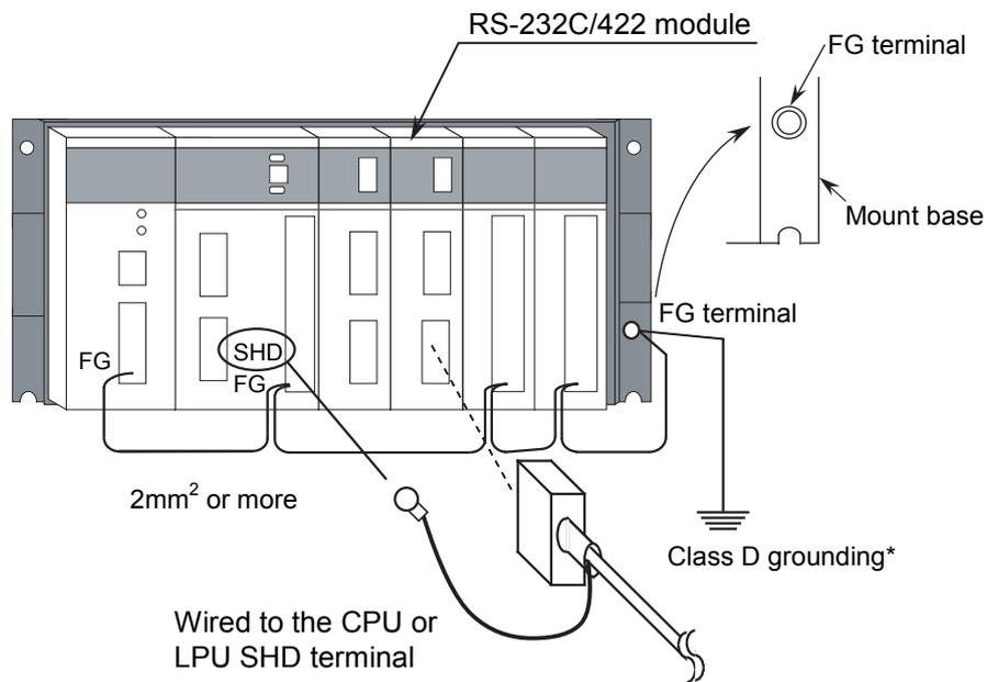
Figure 3-2 Ground Wiring
