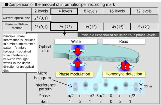
A phase multi-level read/write method is a technology that significantly increases the data capacity of optical discs for archiving video and music. Recording multi-bit (4, 8, 16 or 32 phase levels) information in a single recording mark makes it possible to increase data capacity of optical discs two, three, four, or five times. Data read/write by using four phase levels was experimentally demonstrated.
