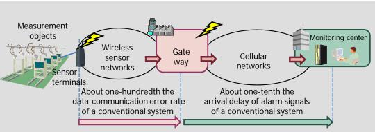
Structure of a remote monitoring system using wireless networks
