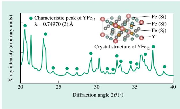
Fig. 4—Constituent Phase Analysis by High-resolution Powder X-ray Diffraction.
