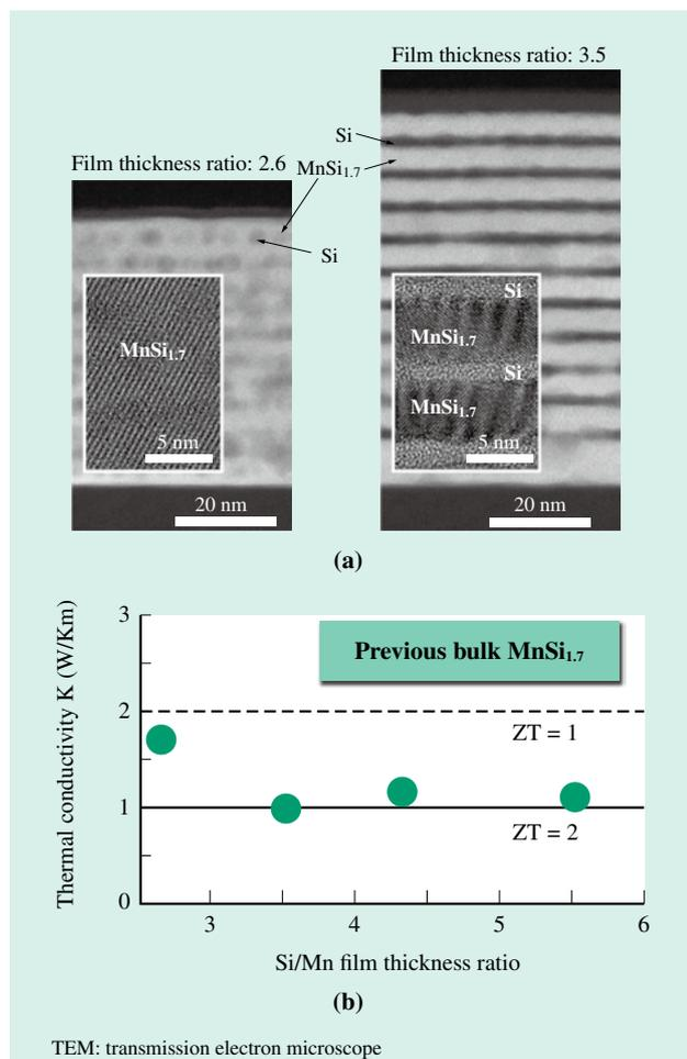
Fig. 2—Cross-sectional TEM Image of MnSi<sub>1.7</sub>/Si Laminate Film and the Dependence of Thermal Conductivity on the Ratio of Si to Mn.
