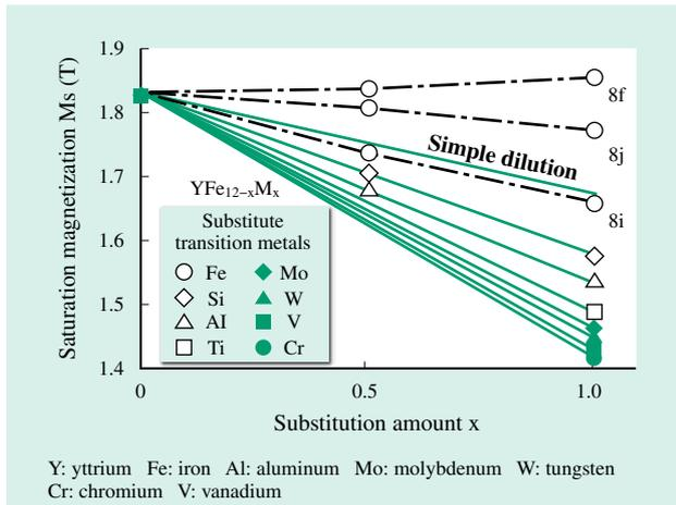
Fig. 3—Dependence (at Absolute Zero) of Saturation Magnetization on Substitution Amount ( $x$ ) Obtained by First-principles Calculation.
