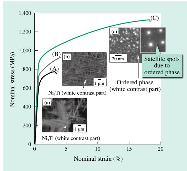
Fig. 5—Tensile Stress-strain Curve and Metallographic Structure for Materials Produced by Casting and by Additive Manufacturing.
