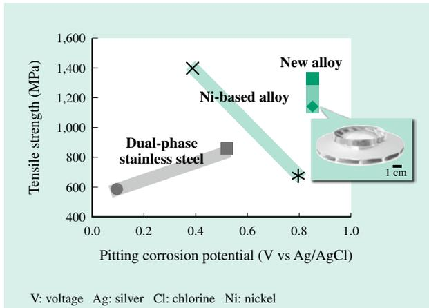
Fig. 6—Comparison of Tensile Strength and Pitting Corrosion Potential in New Alloy and Conventional Alloys. The new alloy has higher strength and corrosion resistance than the dual-phase stainless steel and the Ni-based alloy.
