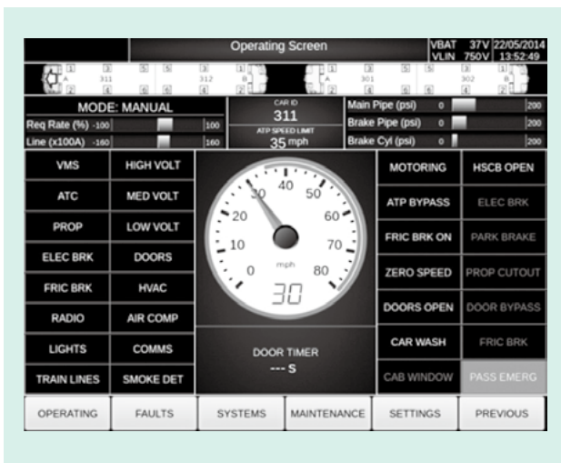
Fig. 5—TOD Layout View. The TOD touchscreen is installed in the emergency driver desk. The layout for diagnostics and alarms is easy to customize to satisfy customer requests.
