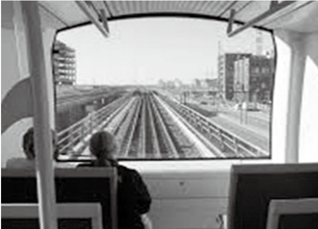
Fig. 2—Front Windscreen. The main characteristic of a driverless train is the absence of a driver cab, instead providing a front large windscreen for passengers.
