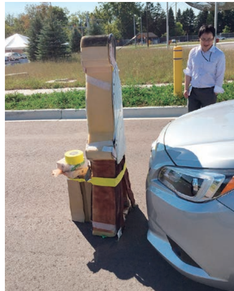
Photo of an automatic emergency brake function test at Mcity
